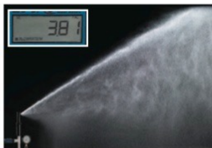
Non-PRS competitive rotor with 3 gpm nozzle at 79 psi inlet pressure. Without PRS, flow rose to 3.81 gpm.
